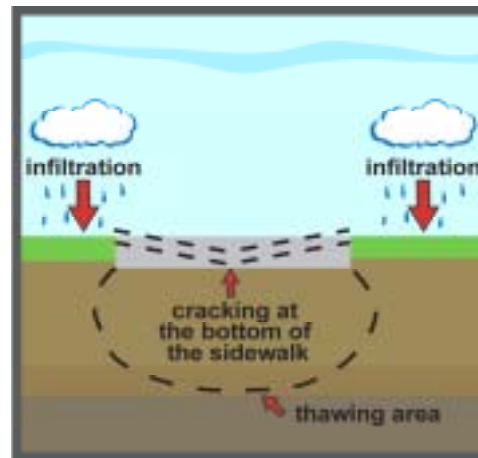
Figure 3–13: Sagging of Concrete Sidewalk
